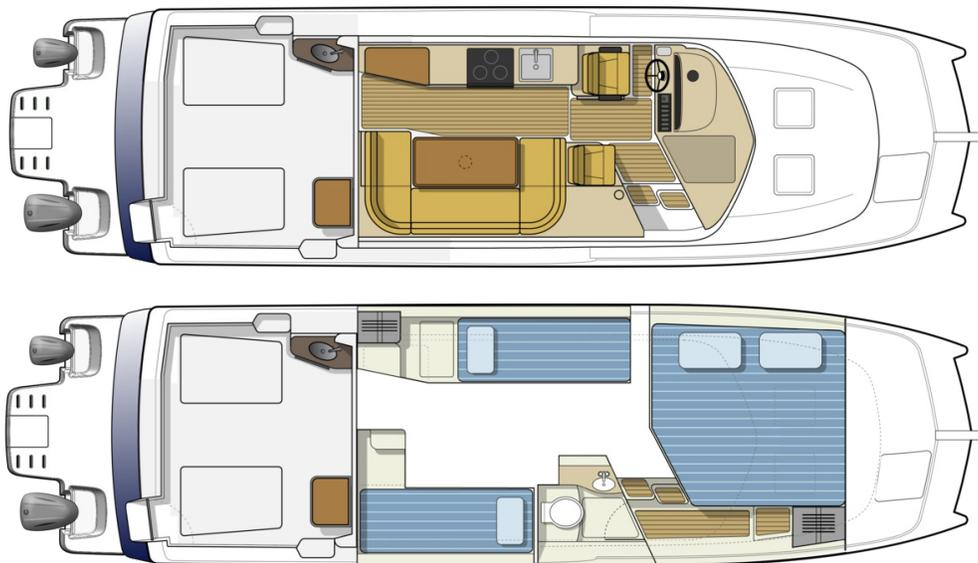
With this new design the overall living space of the new Aspen C108 is increased. New features include a wider salon with a large wrap around dining/seating area, expansive SolarGuard side windows, a larger head, and a second quarter berth, meaning three private cabins.
