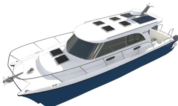
Aspen's new C108 utilizes their proven and patented power proa hull design and is powered by twin asymmetrical outboard motors. The salon is extended 24" from previous interior layouts on other cruiser models, and the
